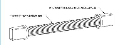
The #6 Secure Mini Dukt™ (SMD) Through-Wall Kit provides a 1" through-wall pathway connecting:
