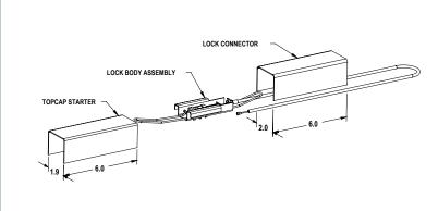
The Steel Raceway Locking Kit is required to securely lock down the Secure Raceway. When in "lock-down" position, the entire raceway is secure and the enclosed cables are protected. Releasing the lock enables the raceway to be repositioned and expanded for future Moves, Adds and Changes. The Steel Locking Kit is used with steel and aluminum Secure Raceway.
