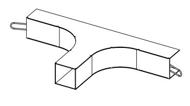
The Internal Three-Way Connector splits the Secure Raceway run, allowing the original run to continue while another run spans across a hallway to the opposite wall. Holocom recently improved upon its original Internal Three-Way Connector by consolidating two pieces into one. The design to a single-piece connector makes installation easier and faster.
