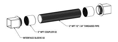
This Through-Wall Kit provides a 2" through-wall pathway from one Secure Raceway section to another Secure Raceway section.
